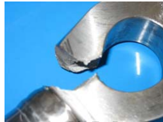
PH-F-158 ROD HEAD BROKEN 76.765 CYCLES AT 308 BAR
