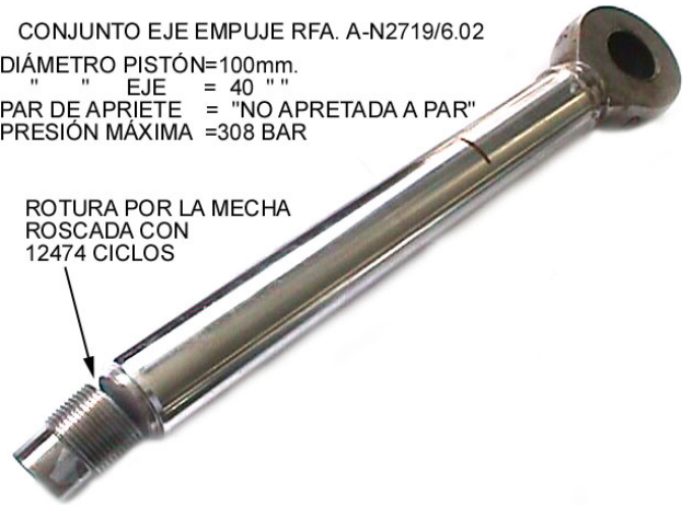
PH-F-158 PISTON END BROKEN 40.991CYCLES AT 308 BAR
