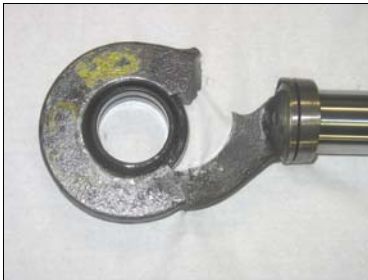
PH-F-179 ROD HEAD BROKEN 125.675 CYCLES AT 308 BAR
